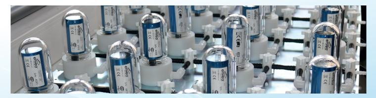
\*Cairsens® sensors are manufactured in France and calibrated in our metrological laboratory using Standard Reference AQMS monitors. Every sensor shipped includes a **calibration certificate**.
